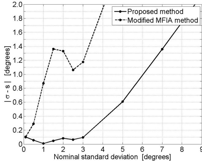
Figure 3: Precision in terms of the absolute difference between the known standard deviation  $\sigma$  and the computed standard deviations.
