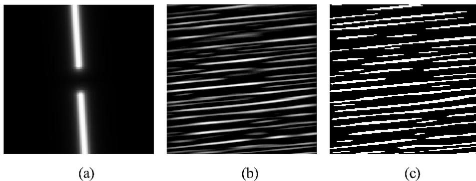
Figure 2: (a) Domain specific Fourier filter. (b) Result of inverse Fourier transformation after Fourier filtering. (c) Binary image obtained with a threshold value and thereby isolating individual fibres as elongated objects.
