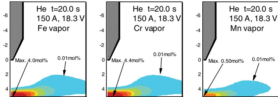
Figure 3: Distributions of iron, chromium and manganese vapor in arc plasma.
