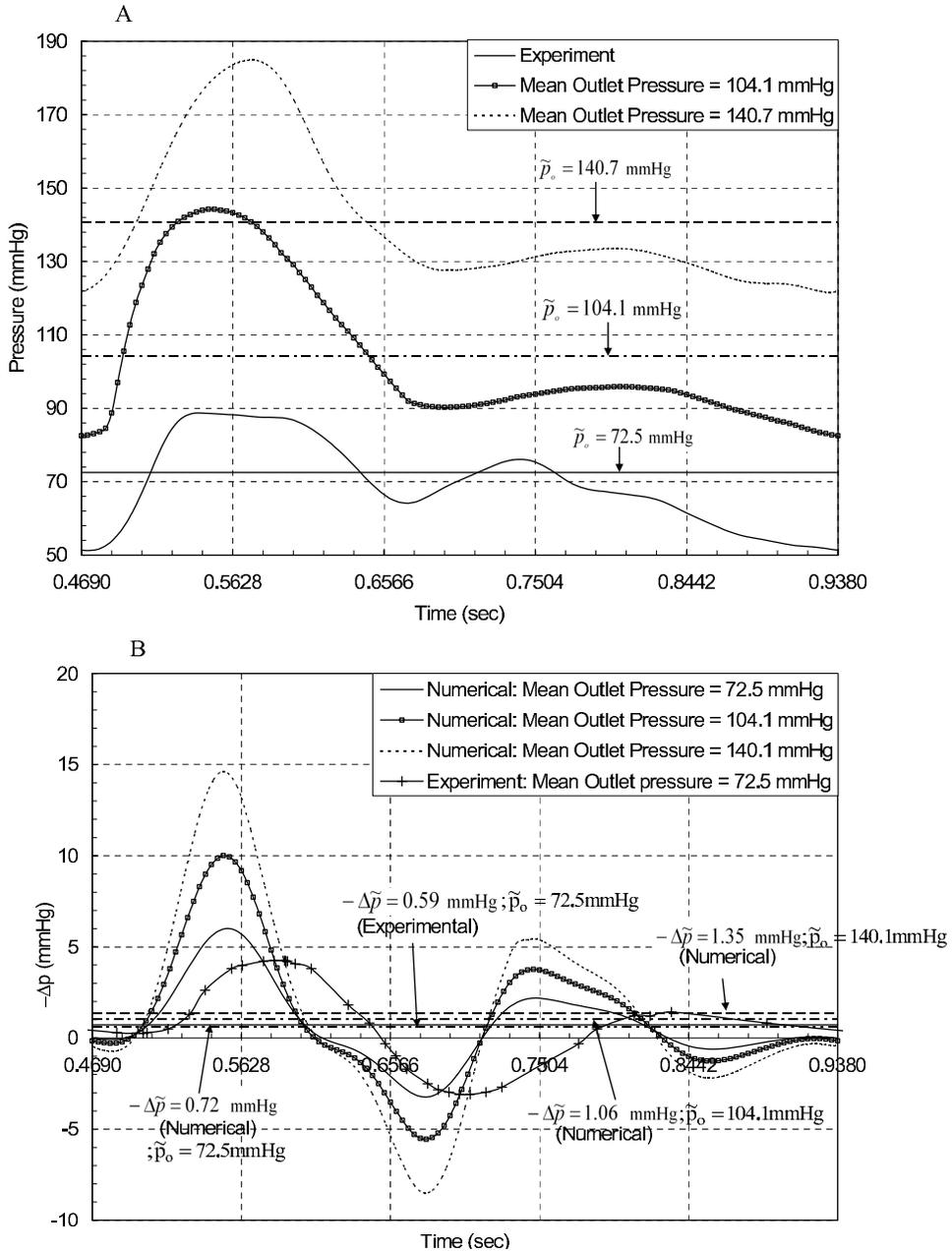
Figure 5: (A) Measured *in vivo* pressure profiles: baseline and elevated; (B) Measured *in vivo* and computed pressure drop between inlet and outlet.
