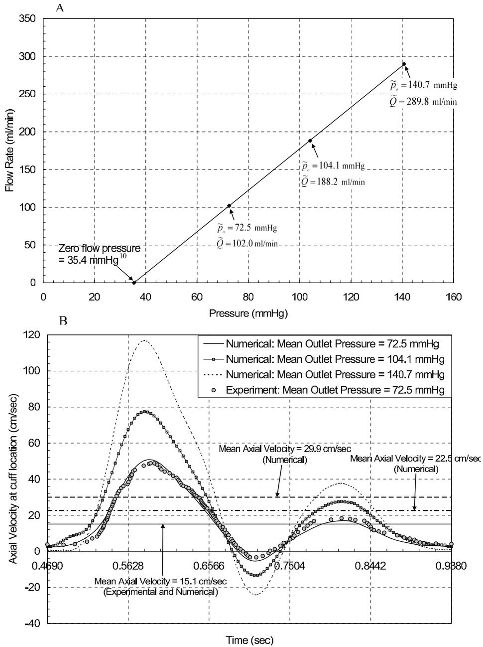
Figure 4: Estimation of flow using linear pressure - flow relationship: (A) Extrapolated linear pressure - flow relationship for baseline and elevated pressure; (B) Measured *in vivo* and computed spatially averaged axial velocity profiles at cuff location.
