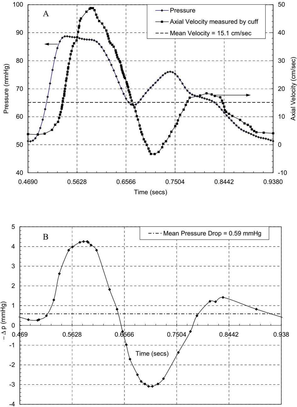
Figure 1: (A) Experimental pressure and axial velocity measured in the tapered femoral artery of dog; (B) Measured *in vivo* pressure drop measured between the inlet and outlet of the tapered artery section.
