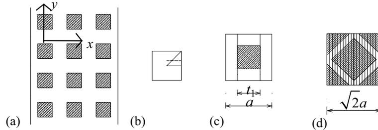
Figure 1: The schematic (a), the first Brillouin zone (b) and the calculated unit cells of the 2D phononic crystal along the high-symmetry lines of the first Brillouin Zone for the  $\Gamma X$  direction (c) and  $M\Gamma$  direction (d).
