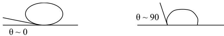
Figure 3: Schematic representation of the nanobubble for T \sim 500\text{K} (left) and T \sim room temperature (right).
