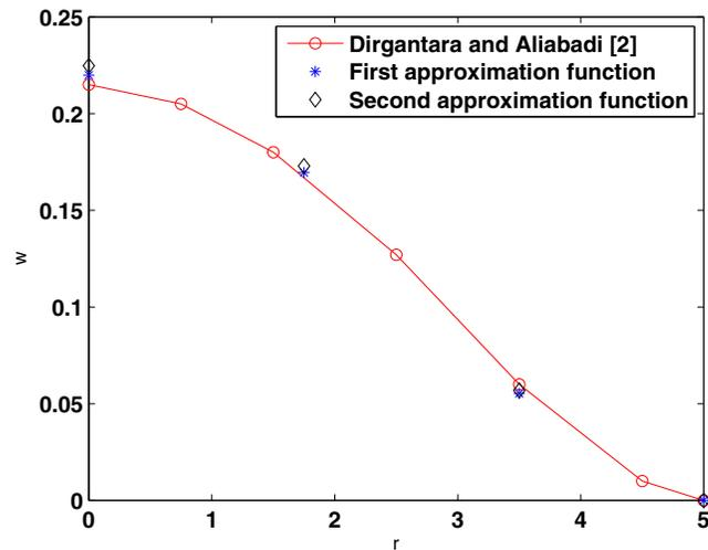
Figure 2: Transversal displacement for the spherical shell with clamped edge.
