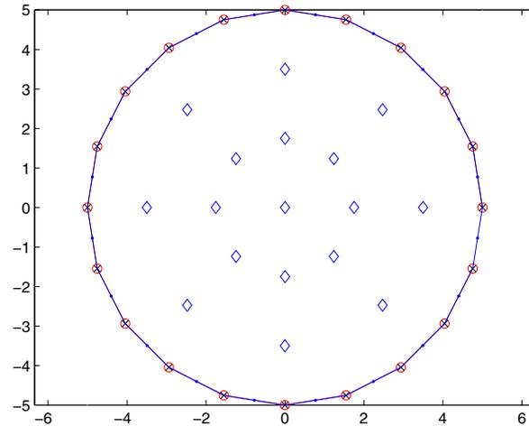
Figure 1: Mesh and internal points for the spherical shell.
