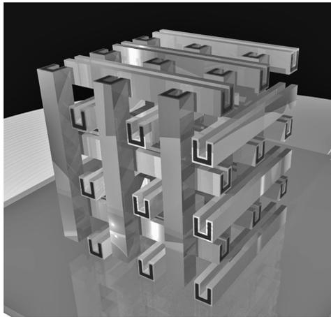
Figure 1: Artist's view of a 3D photonic metamaterial composed of elongated splitting resonators made by DLW of a polymeric backbone and subsequent coating via metal CVD.
