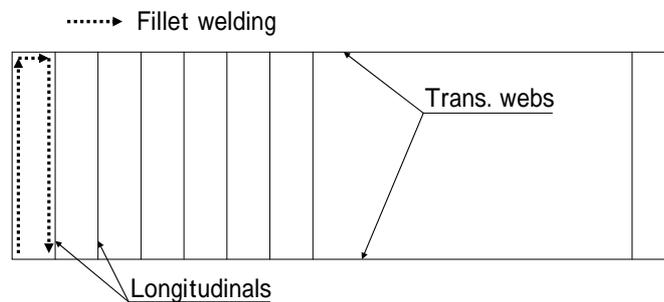
Fig.4 Fillet welding line
