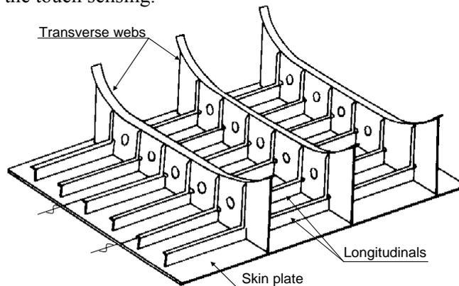
Fig.3 Typical hull block
