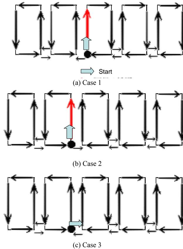
Fig.6 Optimum welding route (1 machine), arbitrary start point
