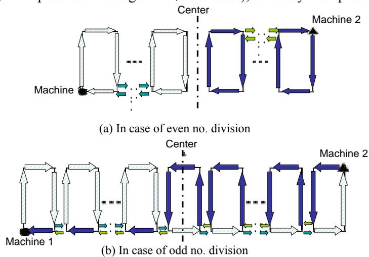
Fig.7 Optimum welding route (2 machines)
