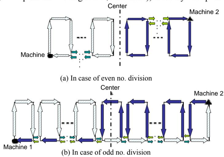
Fig.7 Optimum welding route (2 machines)
