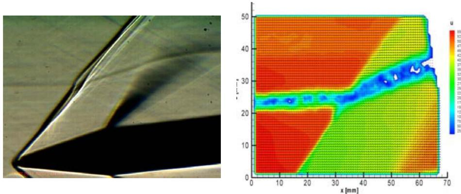
Figure 2: Intersection of a slender longitudinal vortex by an oblique shock at a Mach number  $Ma = 2.2$ , angle of attack of wing  $\alpha_w = 6^\circ$ , and of the shock generator  $\beta_s = 21^\circ$ ; standard schlieren visualization on the left, particle-image-velocimetry results on the right, pictures were taken from [5].
