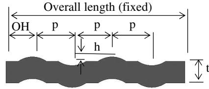
Figure 2: Gasket cross section and design parameters
