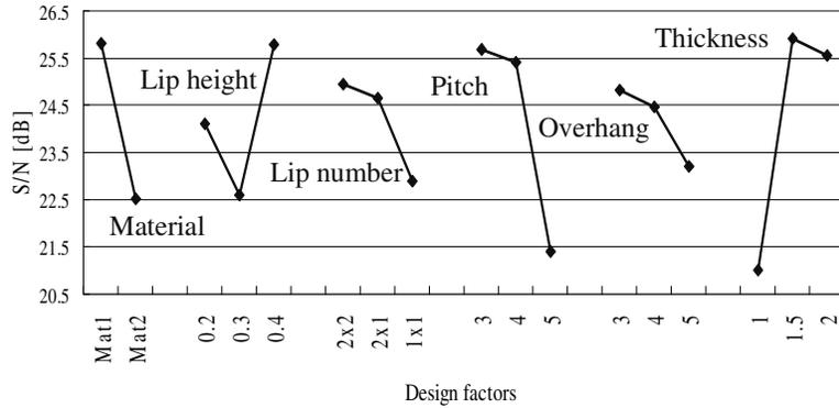
Figure 3: S/N plot: Contact area as evaluation criterion
