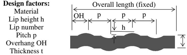
Figure 2: Gasket cross section and design parameters
