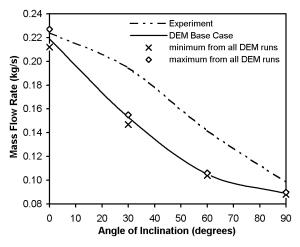
Figure 4: Mass flow rate versus conveyor inclination.
