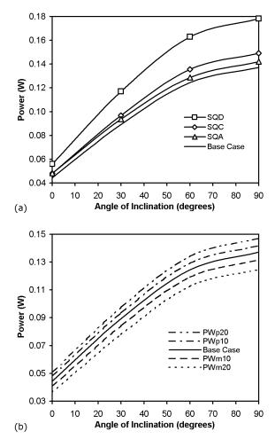
**Figure 6**: Power draw versus conveyor inclination: (a) for super-quadrics particles, and (b) for the full range of particle-boundary friction.
