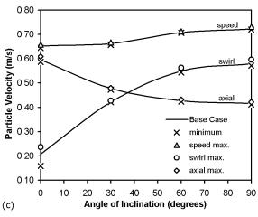
**Figure 5**: Particle velocities versus conveyor inclination: (a) for the full range of particle shapes, (b) for the full range of particle-particle frictions, and (c) for the full range of particle-boundary frictions.
