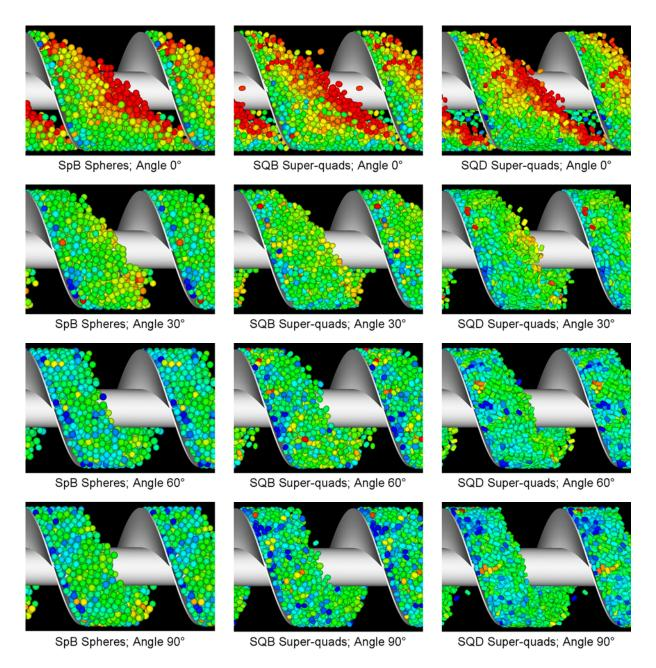
**Figure 2**: Particle flow patterns within the screw conveyor inclined at various angles for different particle shapes. The particles are coloured by their speed: from blue to red for 0.4 to 0.9 m/s respectively.
