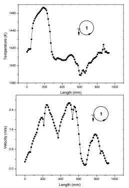
(b) Profiles of temperature and velocity along the specified circle
