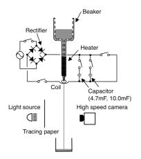
Figure 1: Experimental apparatus for the single pulse electromagnetic force experiment.
