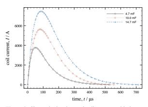
Figure 2: Change in the observed coil currents with time.
