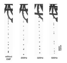
**Figure 6**: Photographs of the formation of the gallium droplets by the intermittent electromagnetic force.
