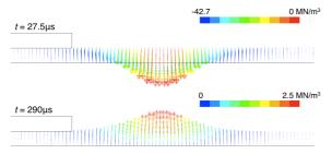
Figure 10: Electromagnetic force field (14.7mF).
