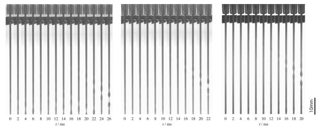
Figure 3: Serial photographs of the breakup of the gallium jet (left: 4.7mF, center: 10.0mF, right: 14.7mF).
