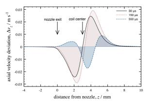
**Figure 15**: Axial velocity deviation from the initial velocity along the center axis.
