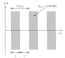
Figure 5: Schematic diagram of the modulated current.
