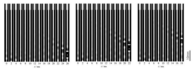
Figure 12: Numerical simulation of the breakup of the gallium jet (left: 4.7mF, center: 10.0mF, right: 14.7mF).
