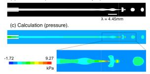
Figure 8: Breakup of the capillary jet by a growth of natural disturbance (without an electromagnetic force).
