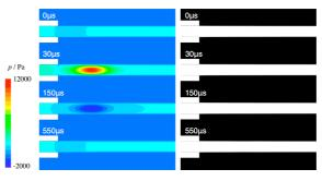
**Figure 14**: Pressure distribution (left) and the free surface of the jet (right) near the coil (14.7mF).
