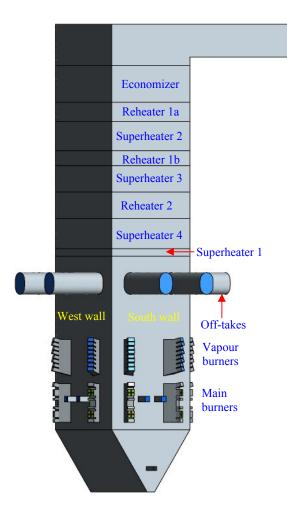
Figure 1: CFD geometry of Yallourn W unit No. 3
