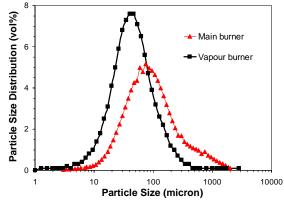
Figure 2: Mill coal particle size distribution at main and vapour burners.
