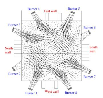
Figure 4: Location of burners and predicted gas velocity vectors for case 1 on plane 1.
