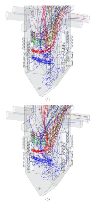
**Figure 8**: Predicted particle trajectories of case 3: (a) with particle dispersion, (b) without particle dispersion.
