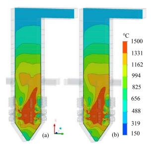
**Figure 7**: Predicted gas temperature profiles of mid-plane: (a) standard k-ε model, (b) SST model, case 2.
