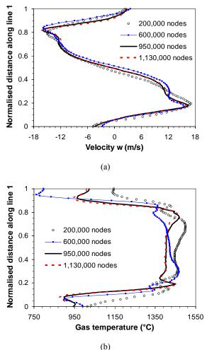
**Figure 5**: Mesh independence test based on (a) gas velocity w, (b) gas temperature along line 1, case 1.
