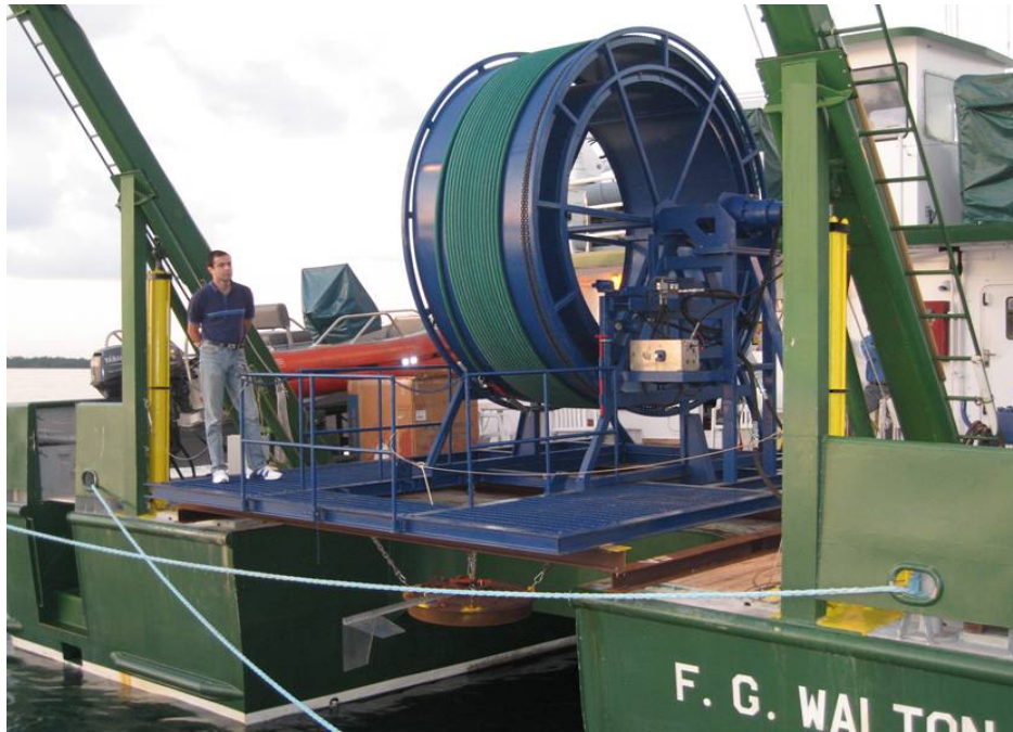
Figure 1. Fiberglass pipe(1.56 cm dia, 153 m long) spooled on the deck of the F.G. Walton Smith. 70 equally spaced, fiber optic, bending strain gauges.
