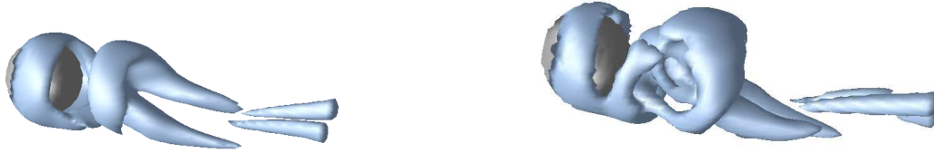
Figure 2: The vortex structure for an isolated particle at Re=300 (left) and Re=600 (right). (Angular view with flow direction from left to right)
