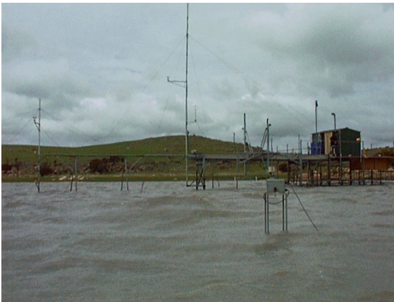
Figure 6. View of the observation platform taken from an offshore location. The two anemometer masts can be seen to the left. The major measurement bridge, where most of the measurements were conducted joins the platform at the right to the anemometer masts. A wave gauge is seen in the foreground.
