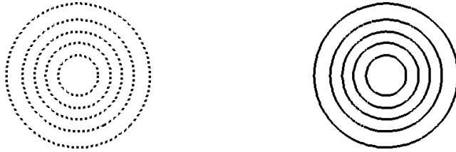
FIGURE 2.3: Contour plot of vorticity for the initial conditions of the 2 vortex system model in two-dimensional space. Contour lines represent unit increments in non-dimensional vorticity. The minimum and maximum vorticity levels were -8 and 8 in the left and right tail vortices respectively. Dashed lines represent negative vorticity levels.
