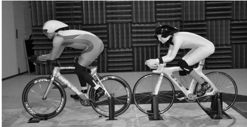
**Figure 2.7.4** - Depiction of the athlete (G) and mannequin in tandem formation at minimum separation distance.
