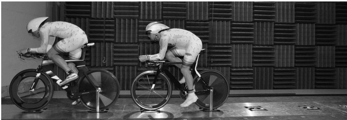
**Figure 2.7.9** - Athletes mounted on Multi-Rider Cycling Rig at minimum separation
