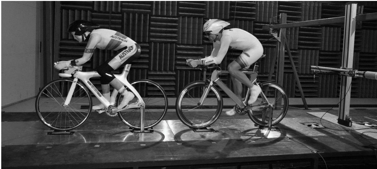
**Figure 2.7.14** - Tandem setup in wind tunnel depicting mannequin and athlete with traverse and probe arrangement downstream of the athlete
