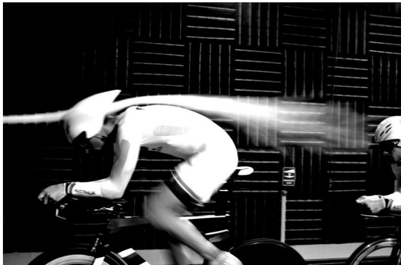
**Figure 5.1.1** - Smoke injected immediately upstream of the lead cyclist's helmet. Athletes in a tandem formation at minimum separation distance (120mm).
