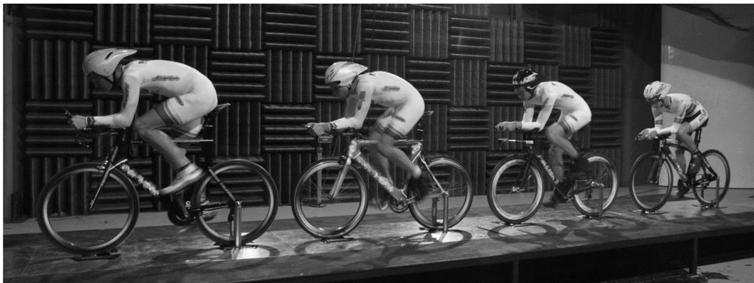
**Figure 2.7.7** - Team formation on rig in wind tunnel test section (displaying Sequence 1 in descending size order)
