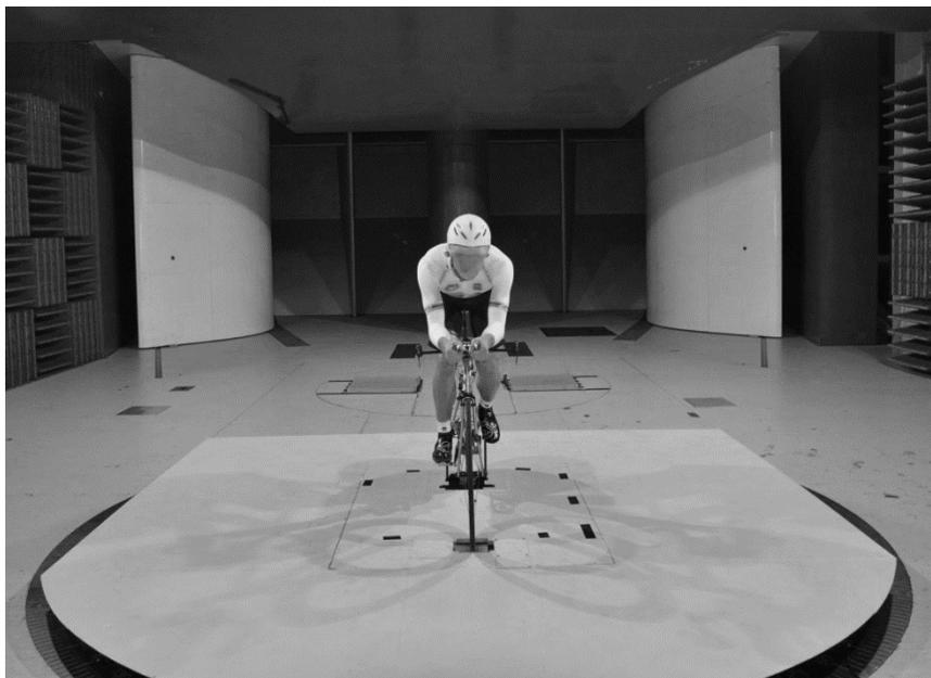
**Figure 2.3.1** - Single Rider Cycling Rig with bicycle mounted on force balance with athlete
