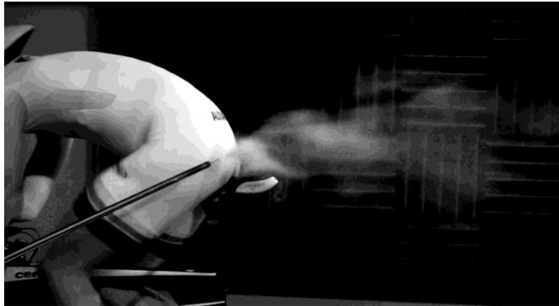
**Figure 5.1.3** - Smoke injected at the hip of the leading cyclist in a tandem formation. Still snapshot taken during athlete pedalling.
