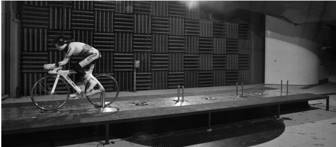
**Figure 2.3.5** - Multi-Rider Cycling Rig shown with mannequin mounted at Position 1. Struts are visible for each of the four force balances that mount at the bicycle rear wheel.
