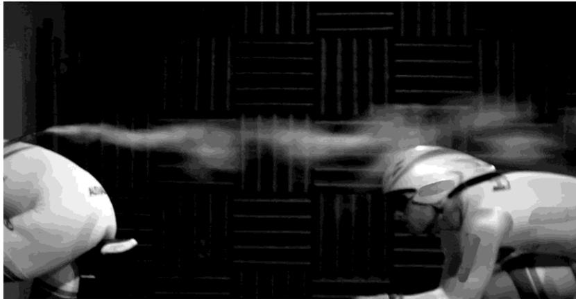
**Figure 5.1.2** - Smoke injected immediately upstream of separation point on the lead cyclist. Riders positioned at minimum separation. Both athletes pedalling during test.
