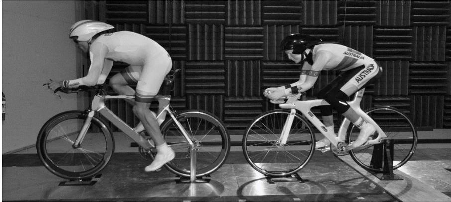
**Figure 2.7.5** - Phase 2 drafting tests conducted on the Multi-Rider Cycling Rig. Depicted here measuring lead rider drag on Athlete B. Mannequin mounted downstream is acting as interference only.
