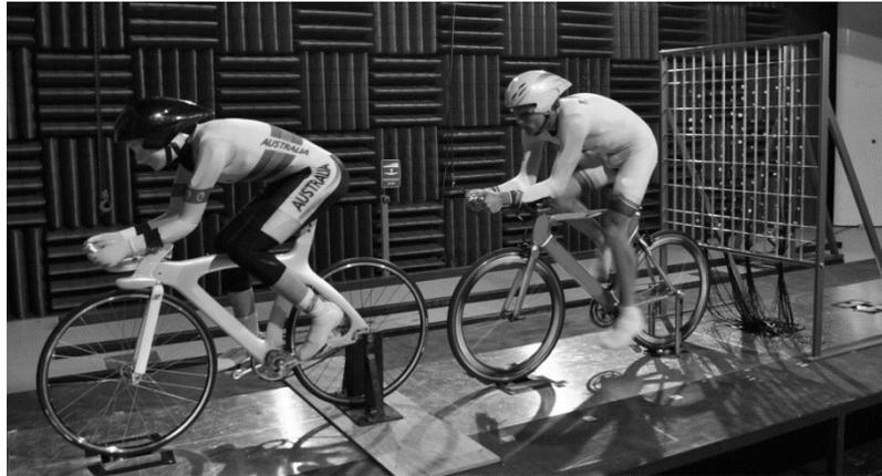
**Figure 2.7.18** - Two rider tandem setup with dynamic athlete in trailing position
