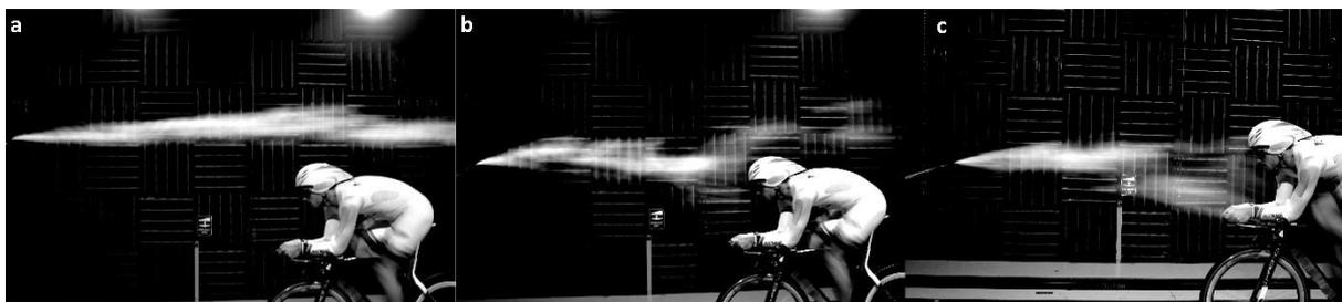
**Figure 5.1.5** - Flow profile ahead of the trailing cyclist at a bicycle length downstream of the lead rider. Three injection points shown, indicated by wand location, highlighting the difference in flow profile with vertical height
