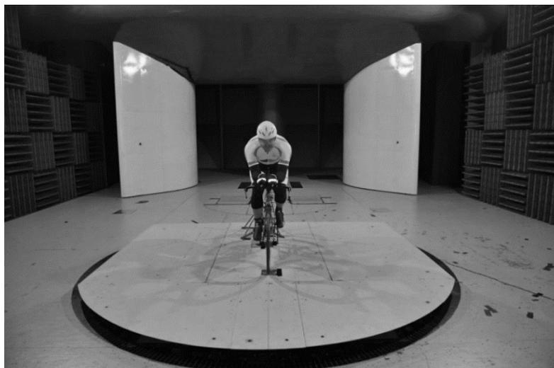
**Figure 2.7.2** – Athlete E mounted on Single Rider Cycling Rig in Monash University Wind Tunnel
