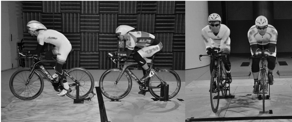
**Figure 2.7.3** – (Left) Riders in tandem formation with instrumented rider trailing; (Right) Riders in side-by-side (transverse) formation with instrumented rider on right of image.
