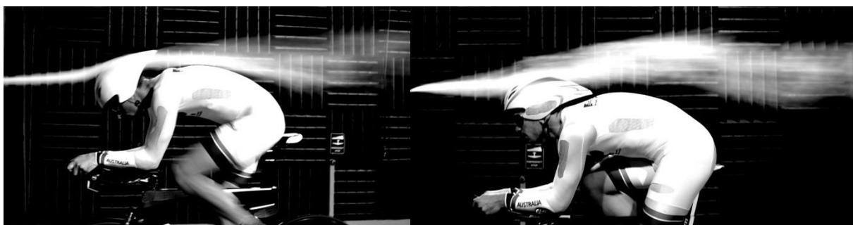
**Figure 5.1.4** - Left; flow over lead cyclist in tandem pair. Right; flow over trailing cyclist with bicycle length separation between riders
