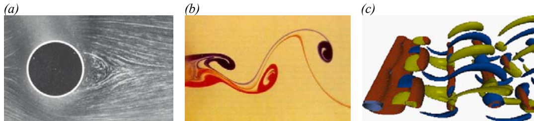
Instabilities developing in the wake of a circular cylinder. (a) The steady two-dimensional wake below Re = 46 (Van Dyke 1982), (b) the periodic two-dimensional Kármán vortex street above Re = 46 , and (c) the three-dimensional “Mode A” wake above Re \approx 190 (Thompson, Hourigan & Sheridan 1996).
